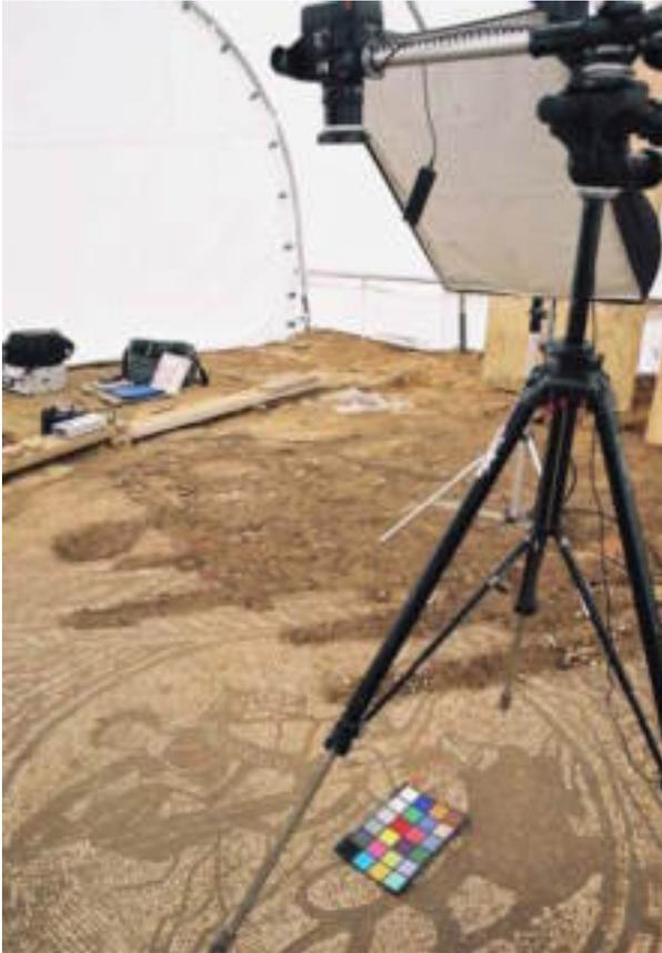
Figure 1 Rolleiflex 6006 semi-metric camera set up on an extension bar with a Macbeth chart in the image.
