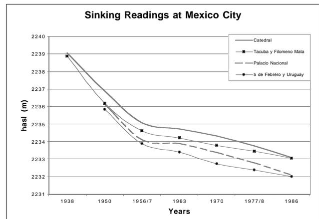
Figure 1. Table of readings of height above sea level through time in four points at downtown Mexico City
