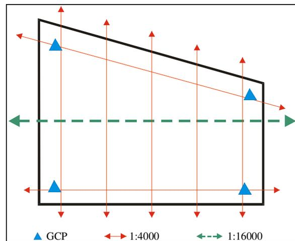
Figure 3. Sketch of the GCPs and flight strips.
