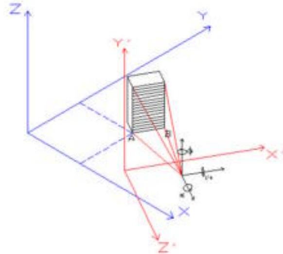
Figure 2. Coordinate transformation form local to photogrammetric reference system
