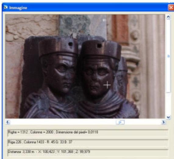
Figure 10. The solid image and the cursor giving the XYZ object co-ordinates of the pointed pixel
