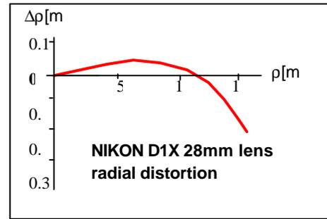
Figure 7. The lens radial distortion curve
