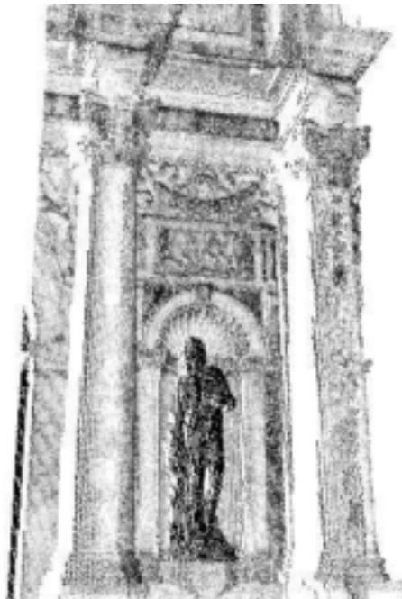
Figure 1 – A DDEM obtained using a RIEGL LMS Z210 laser scanner - Piazza San Marco- Venice – Italy
