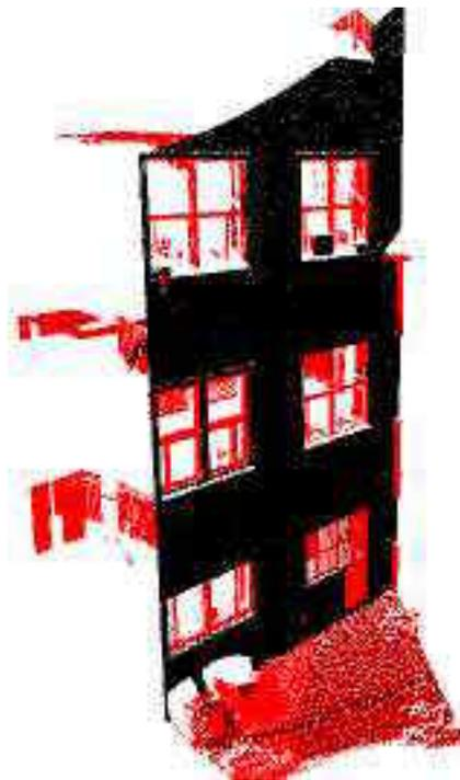
Figure 4 - Segmentation of a building façade. Test area of the Politecnico di Torino – Department of Georesources and Land.
