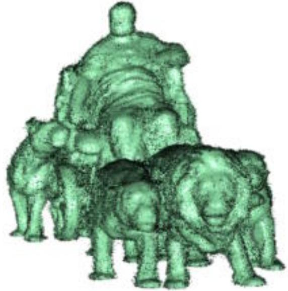
Figure 5: Triangulation of the unfiltered point cloud. Measurement noise leads to a rough surface representation.
