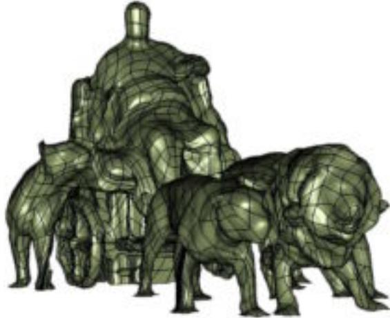
Figure 6: Smoothed surface with automatic generated NURBS patches. The black lines show the patch boundaries.
