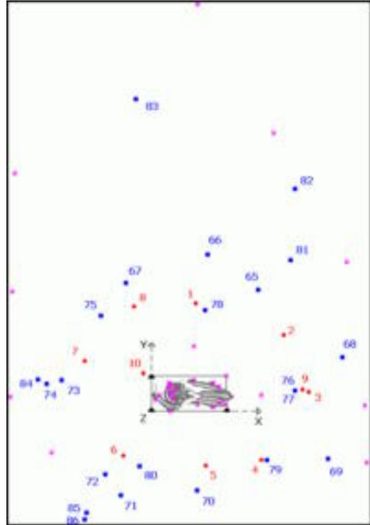
Figure 2: Scanner positions (red circles), photo positions (blue rectangles) and signalized tie points (magenta crosses). The three black triangles on the statue are used to define the global statue co-ordinate system.
