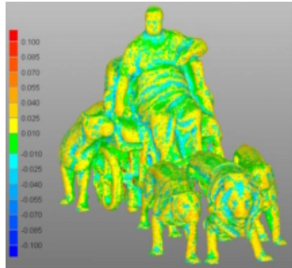
Figure 7: Color coded difference model between the final triangulated surface and the original laser point cloud data (units: m).
