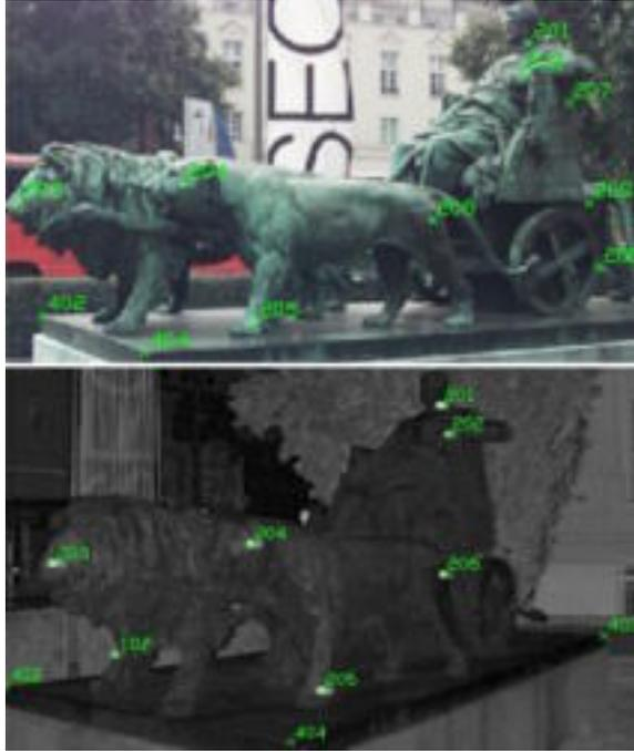
Figure 3: Measurement of tie points (Upper image: photo data, Lower image: Intensity image of the laser scanner).
