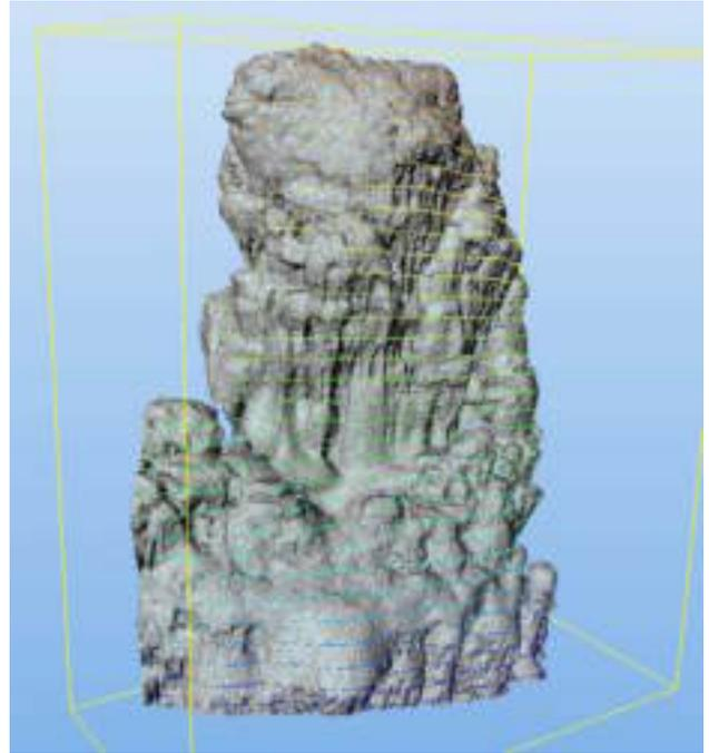
Figure n. 11 3D mesh of the surface and horizontal sections.
