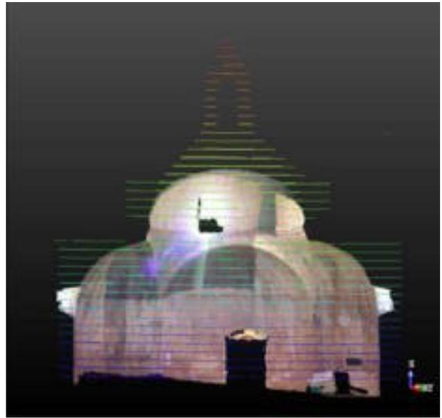
Figure n. 7 The 3D model of the interior surface with RGB.
