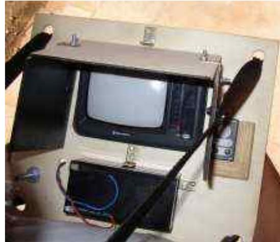
Figure 3. Ground control unit with monitor and remote control
