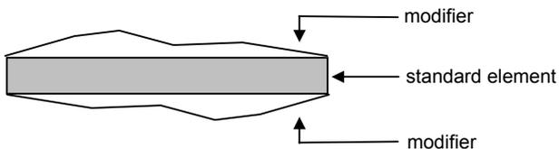
Figure2b. Adaptation of wall surface profile using tacheometric measurements – principle
