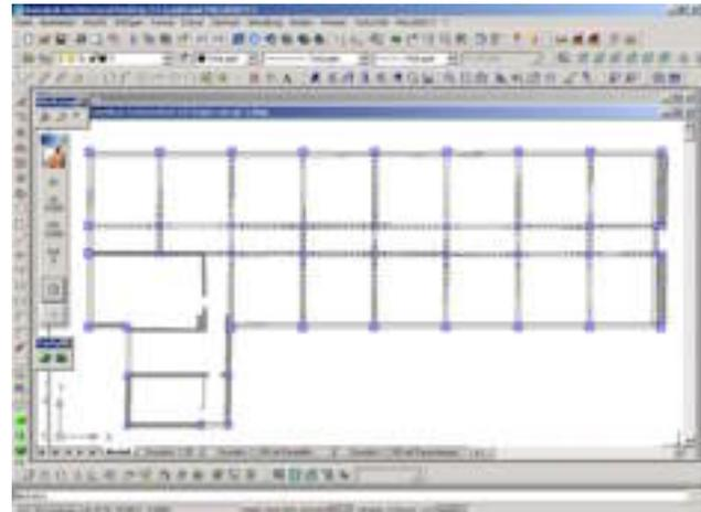
Figure 5a. Plan: Columns, beams, walls
