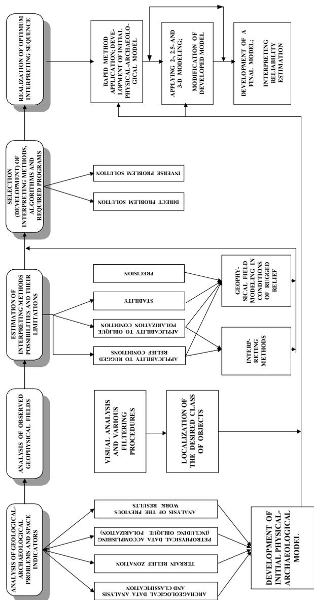
Figure 1. Flow-chart of geophysical data processing and interpretation at archaeological sites (after Khesin et al., 1996, with modifications)
