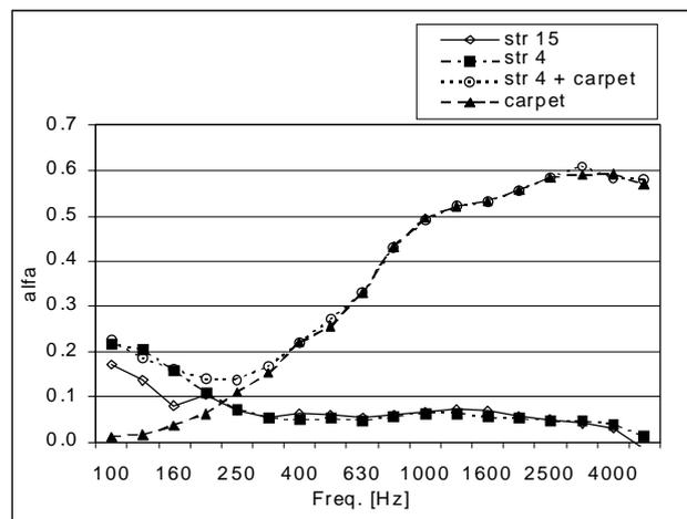
Figure 8. The absorption coefficient for each of the four tested configurations.
