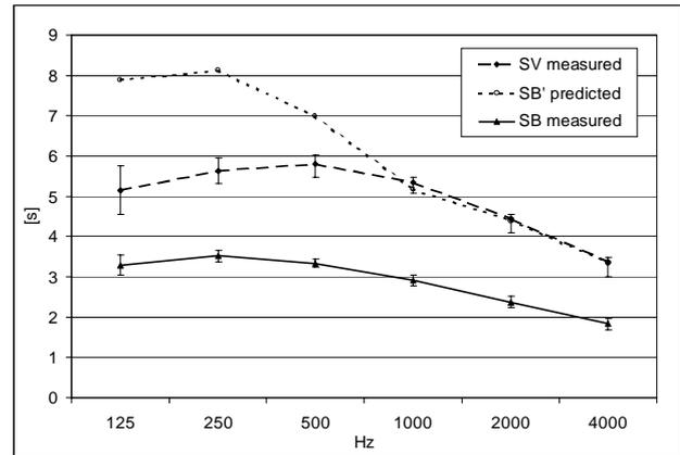
Figure 9. Experimental reverberation time curves for SV and SV and theoretical predictions for SB<sup>ˆ</sup>.
