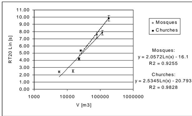
Figure 2. The relationship between the measured reverberation times and the volumes of mosques and churches: all pass values.
