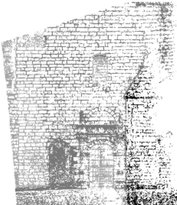
Figure 8. Example of DSM constructed with M1-2 (Pan) pair. There is an empty area (hidden) to the right of the tower.
