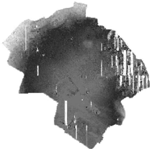
Figure 2. The DTM computed by autocorrelation on the central area of the plateau. Some undulations (or micro-reliefs) are clearly non-natural. The white zones represent lack of data; this is due to the photogrammetric software used for DTM estimation.
