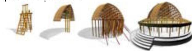
Fig.6: Construction of a Fale Tele
