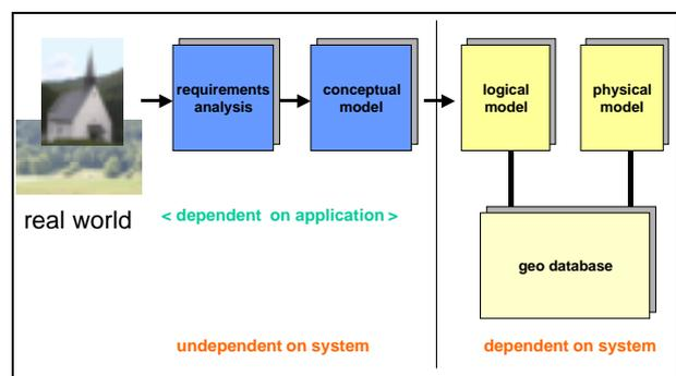
Figure 3. Modelling process from real world into a geo database
