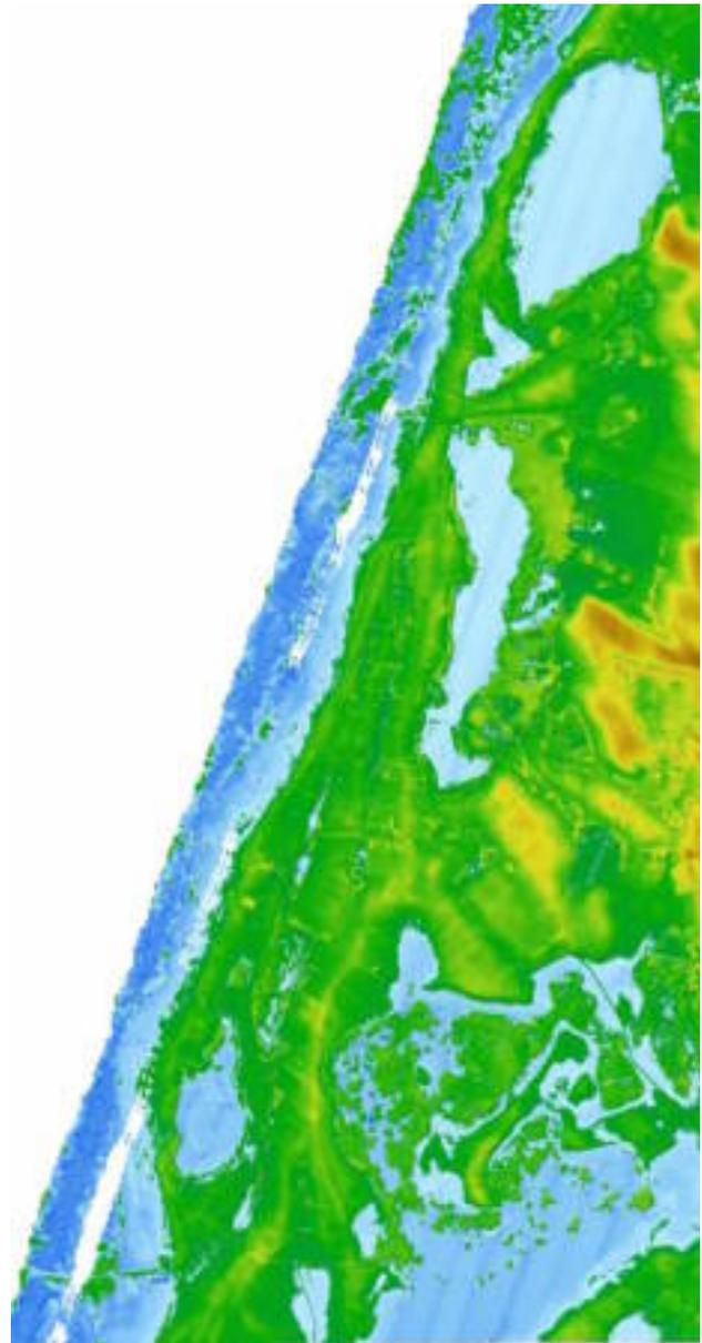
Figure 4: Color coded terrain model derived from laser scanner data.
