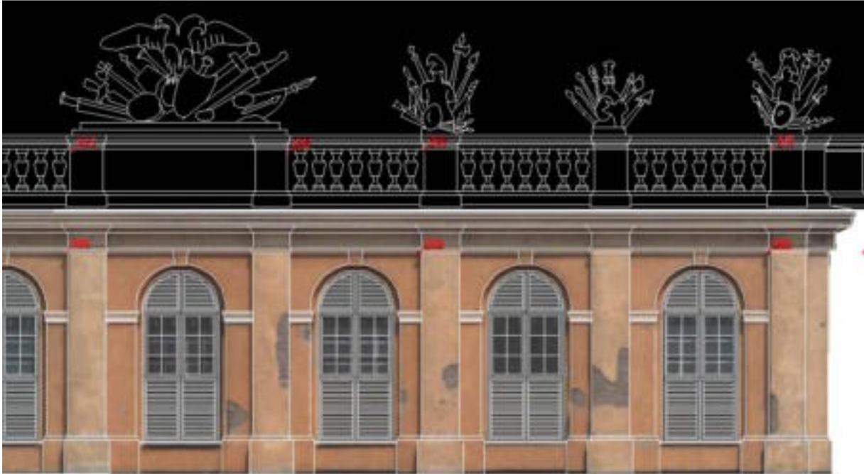
Figure 6: Digital orthophoto of a small section of the facade of the Schönbrunn Castle, with vector data overlaid.
