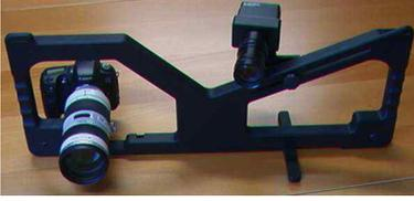
Figure 3: Eyetrionics ShapeCam consisting of a CCD-camera (left) and a flashlight mounted on the top-right part of the handling frame.
