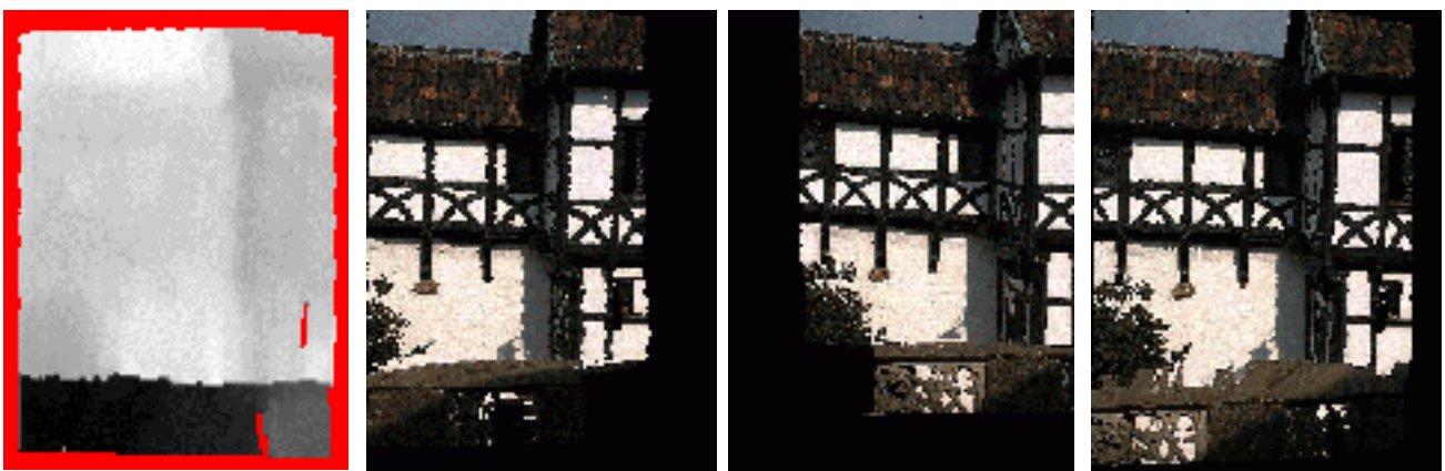
Figure 7: Disparity map (left) and visualizations based on the disparity map
