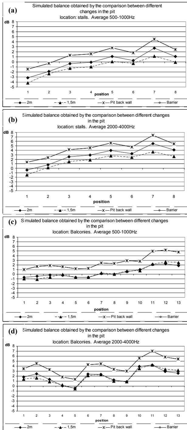
Fig.3 The balance is shown: (a, b) the balance in the stalls at 500-1000 Hz and 2000-4000 Hz; (c, d) the balance in the balconies at 500-1000 Hz and 2000-4000 Hz.
