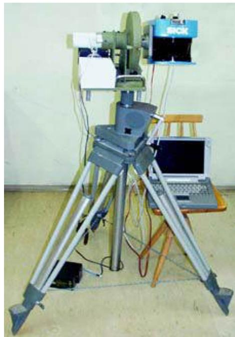
Figure 6. Laser scanner Sick
