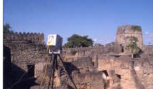
Figure 4 . Laser scanning facing the badly damaged inside walls of the Gereza
