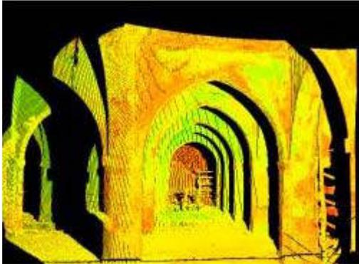
Figure 3 Scan of part of the pillar hall. The pillar scan comprises of 230 000 scan points
