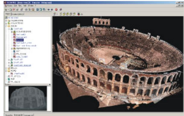
Figure 5: Total view of the online - merged point cloud data from a virtually elevated position (to the right of the image). The color of each point has been taken from the corresponding camera image. To the left the tree structure displays the several scan positions and the files at a single scan position.
