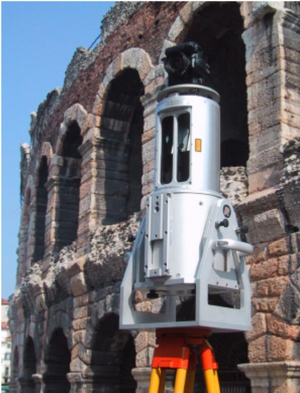
Figure 3: RIEGL LMS-Z360 with Nikon camera mounted on top at work scanning the arena in Verona, Italy.
