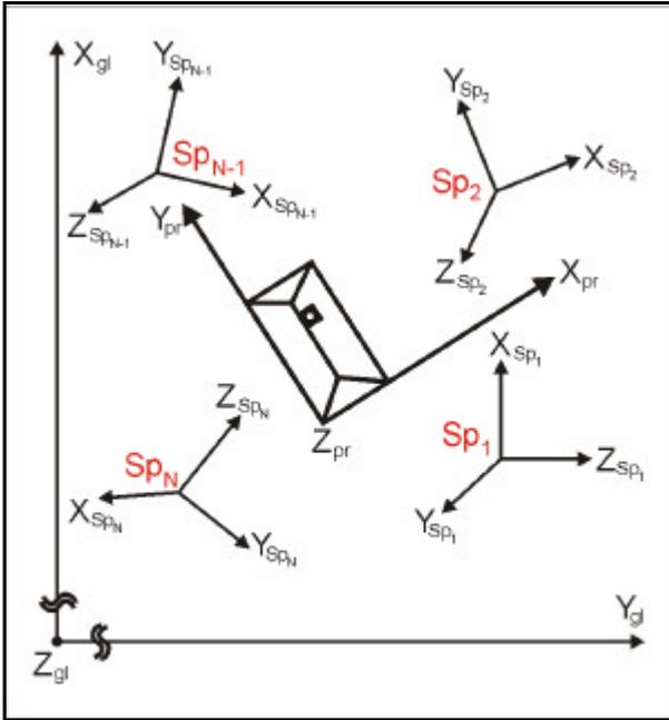
Figure 2: Example for the PRCS, GLCS, and a number of SOCS at a site for scanning a building.
