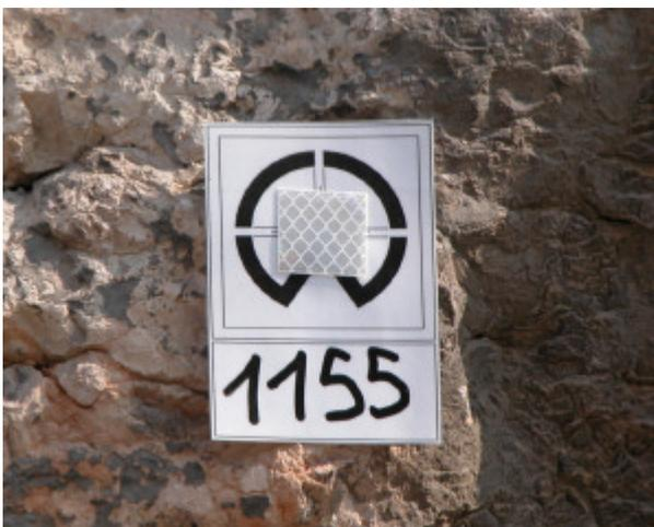
Figure 4: Retro-reflective targets used for merging the scans.
