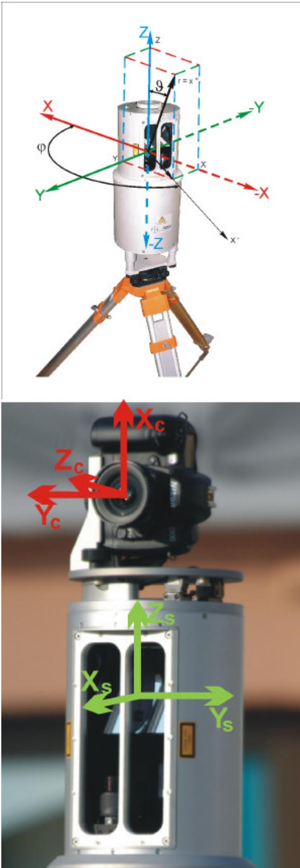
Figure 1: Definition of the coordinate system of a RIEGL LMS-Z360 Laser Scanner (above). Scanner equipped with digital camera mounted on top (below).
