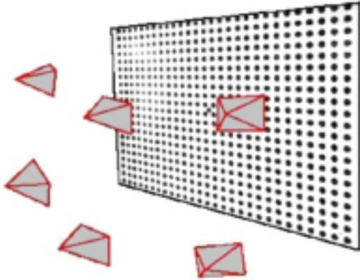
Figure 1: Calibration target for camera calibration. The red pyramids are the camera positions from an exemplary calibration. In the center of the target one can see the marker for automatic registration of the circles.
