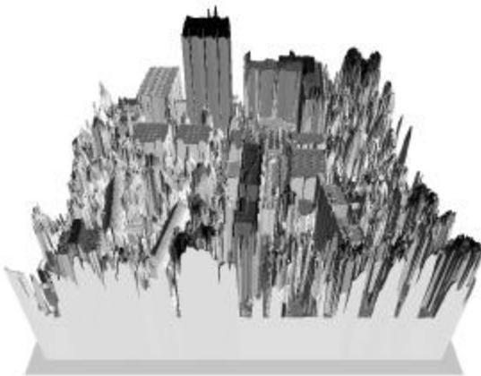
**Figure 1:** 3D visualization of laserscanner derived DEM; first pulse measurement was used
