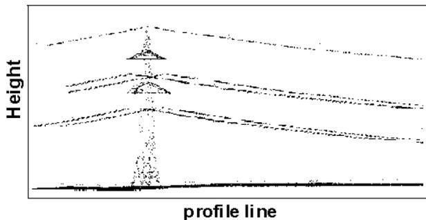
Figure 5: Profile of high voltage power transmission line acquired by laserscanning [Lohr & Schaller, 1999]
