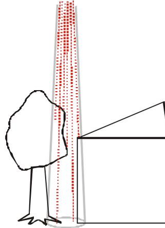
**Figure 2:** Reflection of one laser ray at different objects; outer borders indicated by light grey lines; points show where the signal is reflected
