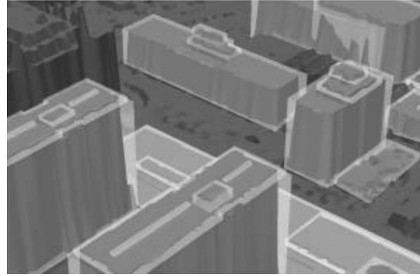
**Figure 8:** CAD- (bright) and last pulse laserscanner- (dark) data
