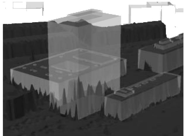
**Figure 9:** Lack in the laser scanner dataset, whole building is missing
