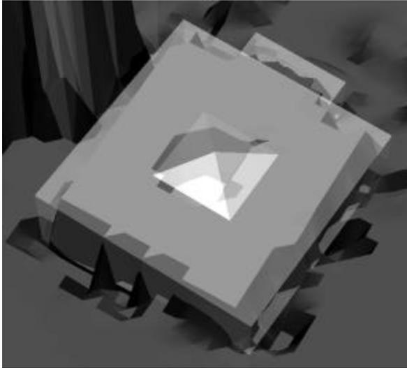
**Figure 10:** Glass pyramide on building, not measured by laserscanning
