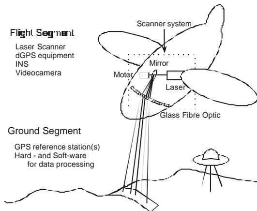
Figure 4: Laserscanner system used by TopoSys company
