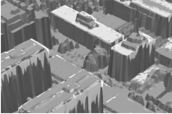
**Figure 7:** CAD- (bright) and first pulse laserscanner- (dark) data
