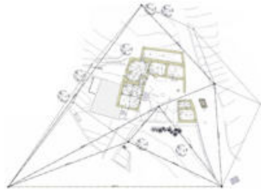
Figure 7. Topographic network and direct survey schema.
