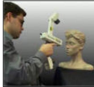
Figure 7: Hand-held laser-scanner HLS (HLS, 2003)
