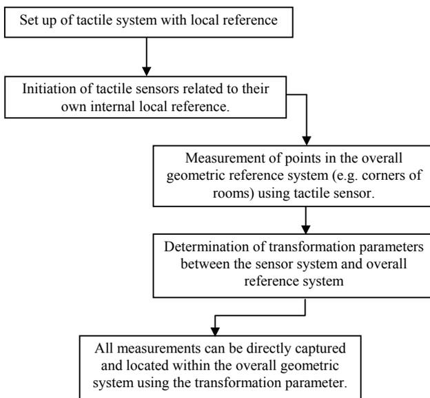
Figure 2: Free positioning of tactile sensors within the overall geometric reference system.
