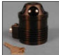
Figure 3: HiBall-3100 optical sensor
