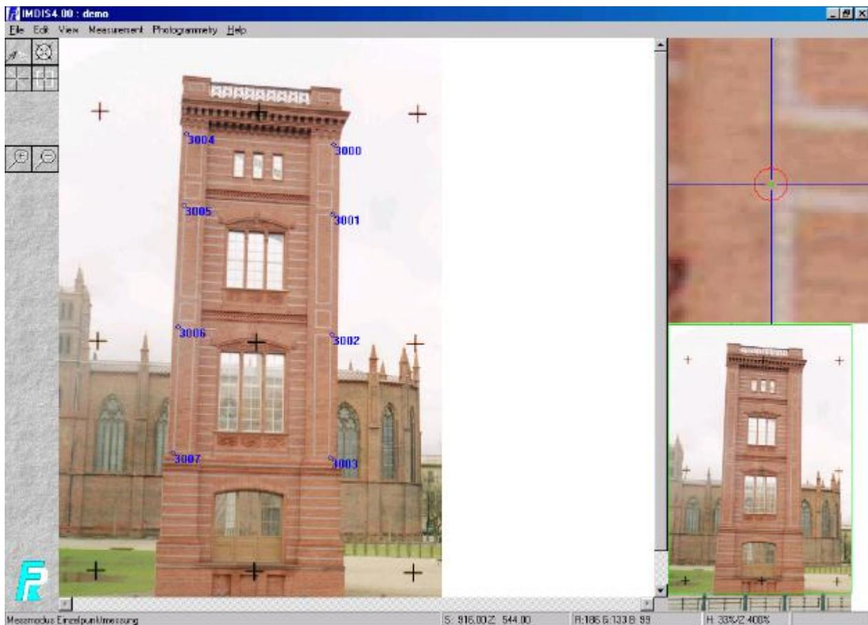
Figure 6: User interface of the IMDIS, the free rectification tool from the Archimedes3D package
