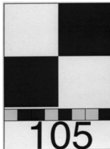
Fig. 1: Point symbol designed for Architectural Survey
