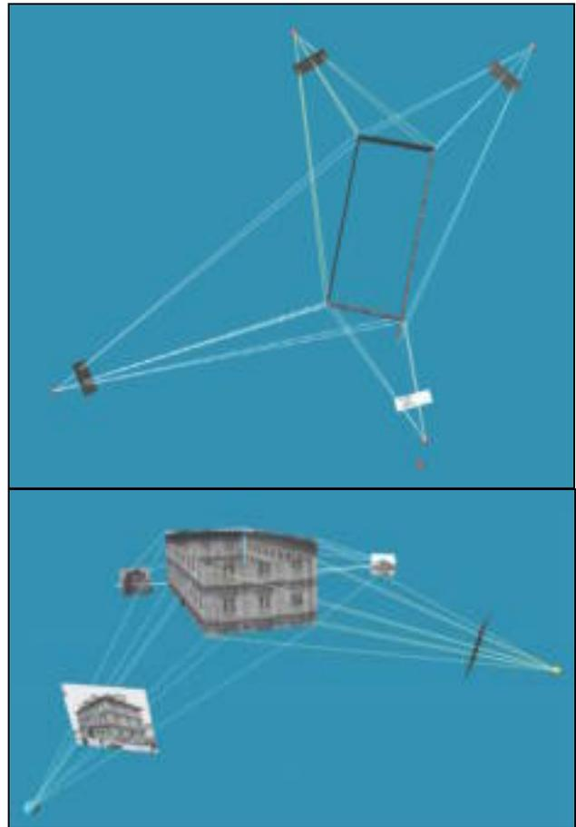
Figure 4: Two views on the approximate reconstruction from the 4 images using the semi-automatic method for orientation
