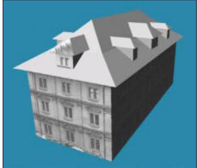
Figure 7: Reconstructed model, partially texture-mapped.
